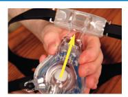
Gently squeeze the sides of the StabilitySelector and slide the arm upward to set the forehead support arm to its highest position.
